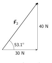
$F_{2x} = (50.00 \text{ N}) \cos 53.1^{\circ}$ = 30 N  $F_{2y} = (50.00 \text{ N}) \sin 53.1^{\circ}$ = 40 N
