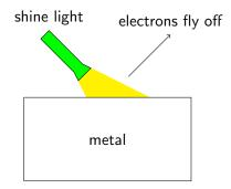
Light provides the energy needed to free electrons from the metal.
